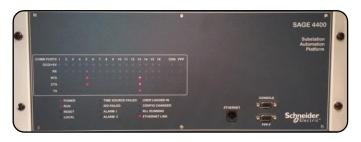
capability and is designed for applications that require a significant capability for discrete I/O along with processor power for integration of many IED's as well as "intelligent" embedded applications and logic functions. The SAGE 4400 is mounted in 19" rack mounting relay style aluminum enclosure with serial and Ethernet communications ports built-in but also provides the capability to have many analog, status, accumulator and control outputs from hard-wired discrete I/O field connections.
