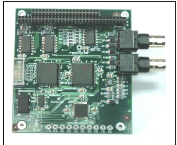
The PC104 IRIG-B Input/Output Module is easy to add to any unit. Simply plug it into the PC104 bus on the existing unit. It is added in the same way that the CPU, Serial Communication Expansion module or the GPS module is added to the PC104 stack. Once the card is added, connect your IRIG-B signal source and/or output to the BNC connections on the IRIG-b card.
